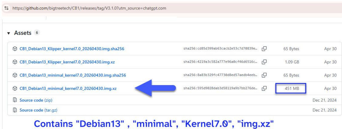
Figure 1. Select the 451MB Debian 13 minimal image—not the Klipper image.
